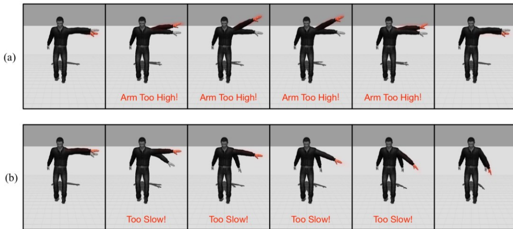
Figure 10. Examples of textual and visual guidance. The rendered red arm shows the user's left arm movement relative to the avatar instructor's, after motion data alignment using proposed GB-DTW technique. Textual guidance is provided on the bottom. (a) The user's arm is higher than required. (b) The user moves more slowly than the avatar instructor when moving his arm down.
