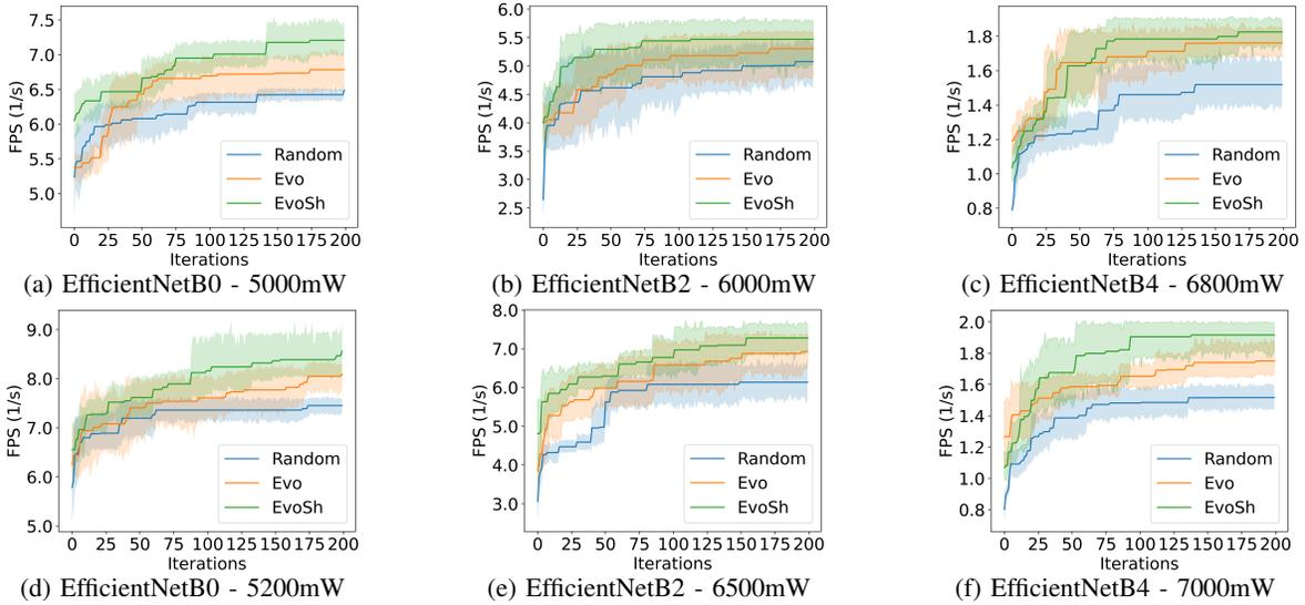
Fig. 4: Performance of search algorithms for different deep learning models with different power thresholds
