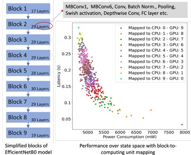
Fig. 1: The search space overview of 9-blocks EfficientNetB0
