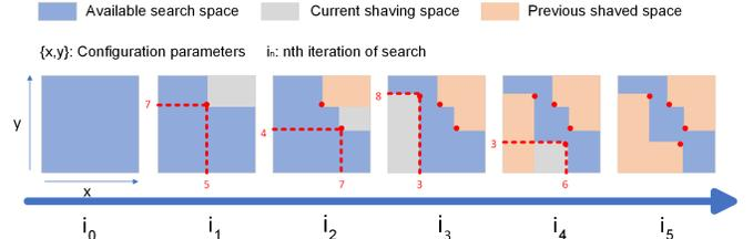
Fig. 2: Two dimensional shaving technique illustration
