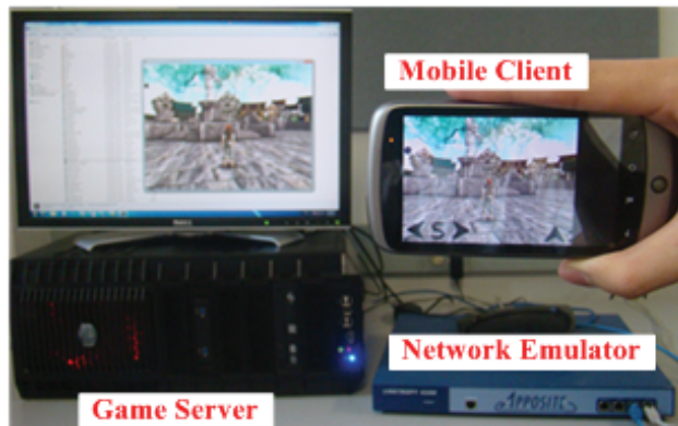
Fig. 4. Test bed of subjective quality assessment experiments
