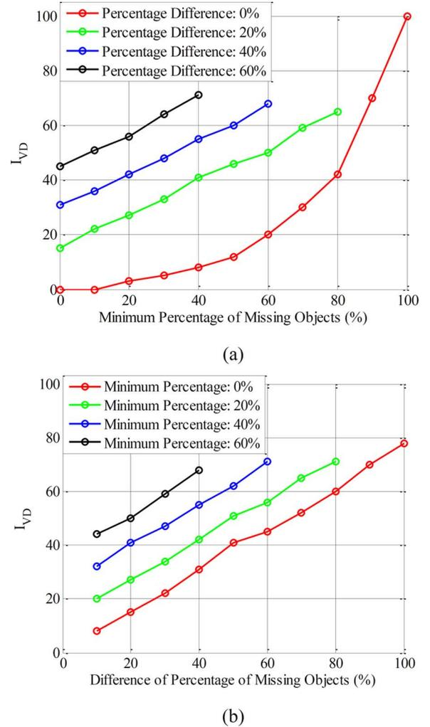
Fig. 6. Subjective test results: (a) top, Relationship between Impairment values and Minimum Percentage of Missing Objects (b) bottom, Relationship between Impairment values and Difference of Percentage of Missing Objects.
