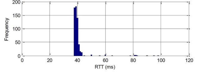
Fig. 16. RTT measured from AWS to test device.
