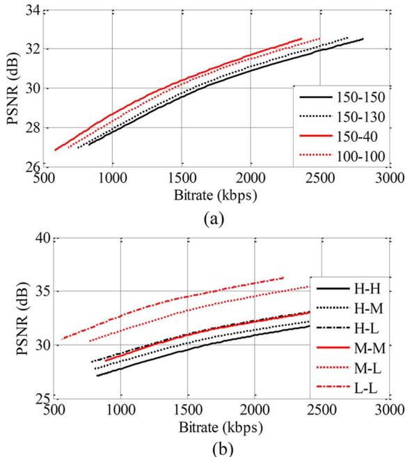
Fig. 4. (a) top, Rate-distortion performance with different view distance setting for left view and right view (b) bottom, Rate-distortion performance with different texture detail settings for left view and right view.
