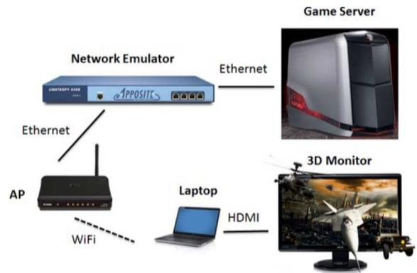
Fig. 5. Testbed for Subjective Experiments.
