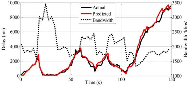
Fig. 14. Results showing actual and predicted delay.
