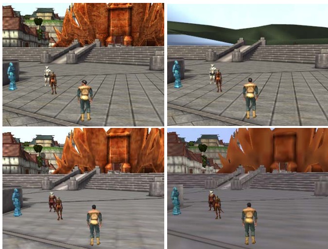
Figure 3. Screenshots of game “PlaneShift” in different settings of view distance and texture detail (LOD): (a) top-left, 300m view and high LOD; (b) top-right, 60m view and high LOD; (c) bottom-left, 300m view and medium LOD; (d) bottom-right, 300m view and low LOD;
