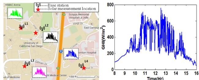
Figure 1. (a) left, Map showing locations of 4 BSs and nearby solar irradiance measurement, (b) right, solar irradiance at L1 on Dec. 11, 2014 between 8AM-4PM
